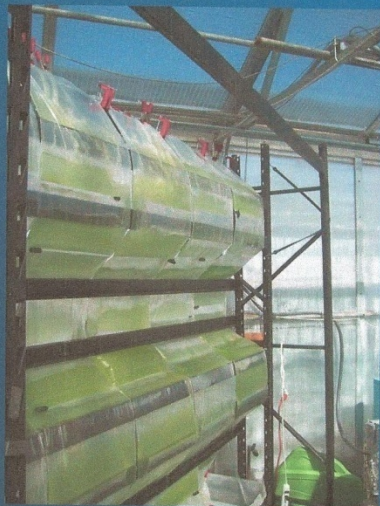
Accordion Photobioreactor (University of Arizona)
